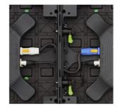
The power and video cables between two modules slot neatly into the 62 mm thickness.
