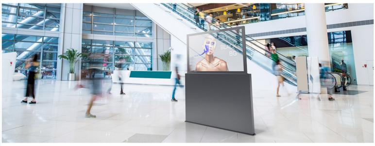
The Innovate Transparent Series is a brand-new type of solution, which makes it possible to achieve transparency without a backlight. The 55" Transparent OLED consists of self-emitting diodes which can operate in any inside environment. Without the need of a backlight or showcase, the Innovate Transparent see-through OLED screen can be placed in the middle of a room or integrated into a wall creating a UNIQUE customer experience!
