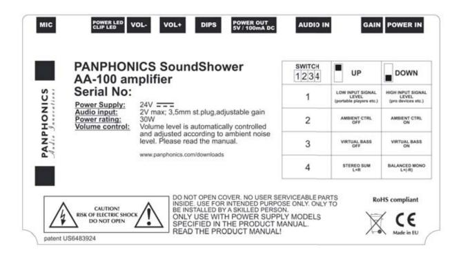
The media source is connected to the Audio IN socket with a 3,5 mm stereo jack. The source maybe any audio source with output level from 50mV to 2V. Typical sources can include devices like any portable mp3, computer, CD etc. For the best audio quality and to avoid any possible electrical disturbances, it is recommended to use a 1,5 m (5ft) long input cable at maximum. External 24V DC power source is connected to the Power In connector. Use only the power supplies provided by Panphonics Oy.
