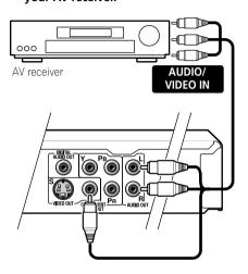
The diagram shows standard video connections, but you can alternatively use the S-video or component video connections if they're available.
