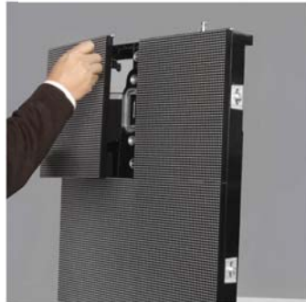
Horizontal pull (Magnetic design)
