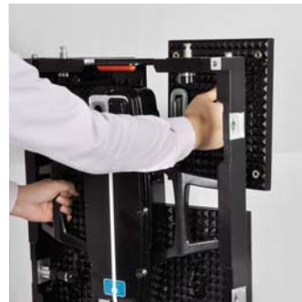
Move the module from front (Magnetic design)
