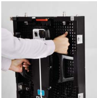
Fasten the module handle and horizontal push
