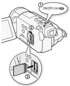
• To use the wireless communication features of an Eye-Fi card, insert it into memory card slot **B**. Be sure you understand the information provided in *Eye-Fi Cards* (C 36) before using an Eye-Fi card.
